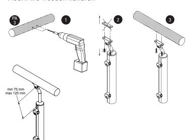
Drilling template for wooden handrail
